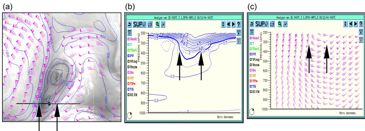
**Fig. 4. Dynamic interpretation of radiances in MSG WV channels. (a) Meteosat-8 image in 6.2  $\mu\text{m}$  superimposed by the 1.5 PVU surface heights. Vertical cross sections (data from ARPEGE) of (b) potential vorticity and (c) wind along the black line shown in (a).**
