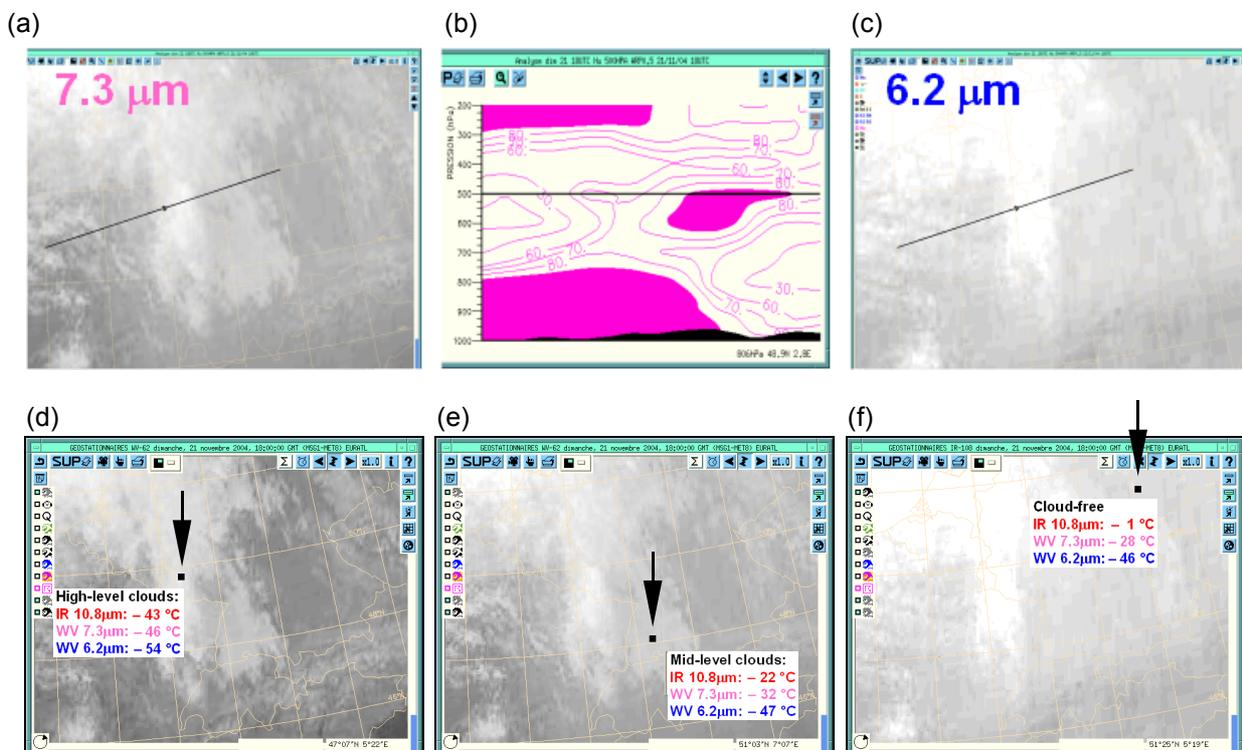
**Fig. 2. Deep moist layers (200-1000 hPa) as seen in MSG WV channels (a) 7.3  $\mu\text{m}$  image. (b) Vertical cross section (data from ARPEGE) of relative humidity (%) along the black line depicted in (a) and (c). (c) 6.2  $\mu\text{m}$  image. Brightness temperatures derived by MSG**
