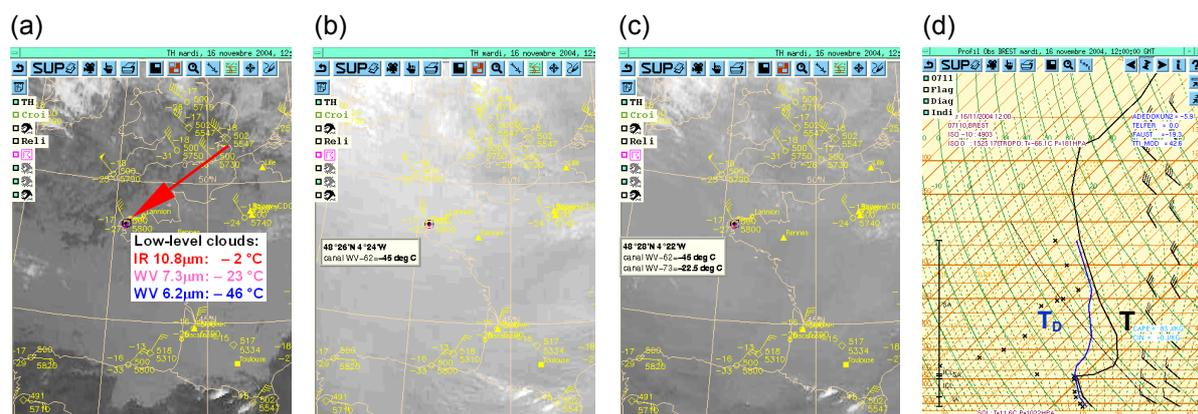
**Fig. 1. Meteosat-8 images in: (a) IR 10.8  $\mu\text{m}$ , (b) WV 6.2  $\mu\text{m}$  and (c) WV 7.3  $\mu\text{m}$  channels. (d) Upper-air sounding at Brest, T - air temperature (black curve),  $T_D$  – dewpoint (blue curve). Also shown the brightness temperatures derived from the three channels at location of the release point of the sounding shown in (d).**
